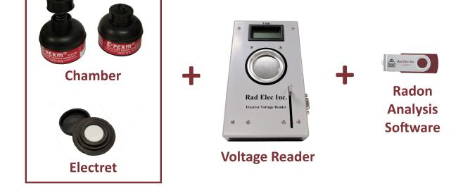
These components are needed to make both short-term and longterm radon measurements, and can be used either indoors or outdoors. When an electret is loaded onto an ion chamber it is called an E-PERM<sup>®</sup>, which is also referred to as an electret ion chamber (EIC).
