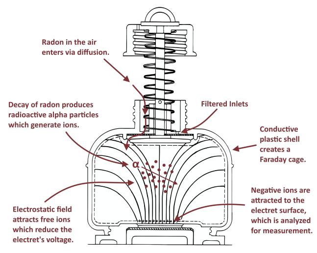
Radon gas (and **not** the progeny present in the air) diffuses through the filtered inlets into an electret ion chamber. This diffusion continues until the radon concentration inside the chamber is equal to the radon concentration outside (typically a room). Radiation emitted by the decay of radon and its progeny formed inside the chamber ionizes the air, which produces both positive and negative ions.
