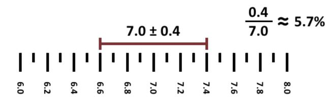
After calculating uncertainty in this specific example, we can be confident that our measured radon concentration is within approximately 6% of the *actual* radon concentration. This percentile value can be calculated after dividing the absolute uncertainty by the measured radon concentration. Uncertainty is calculated automatically when using any of Rad Elec's analytical tools, but this section dives into the math behind this process.
