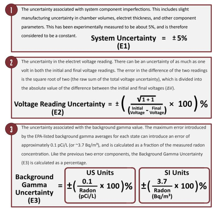
These three uncertainty components can be combined in order to create the **total uncertainty**, or total error, of a specific E-PERM<sup>®</sup> radon measurement. It can be determined by calculating the square root of the sum of the squares of the three individual error components. This is shown by the following equation.
