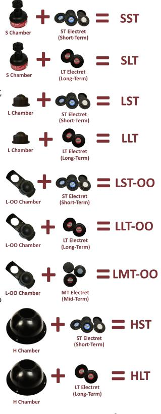
more greatly affected by the decay of radon. This means that very sensitive configurations, such as the HST (H Chamber + ST electret), are intended to measure a standard environment for a short time period (such as 8 to 24 hours). Alternatively, the HST configuration can be used to measure a low concentration environment over a few days.
