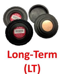
volts. Electrets with fewer than 100 volts exhibit a weaker electrostatic field which is not as consistent in collecting ions efficiently. However, these lower voltage electrets can function as excellent field blanks (recommended for good QA/QC practices) and when fully discharged can be returned to Rad Elec for credit.
