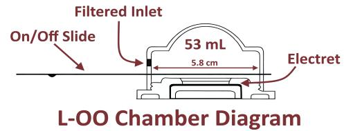
amount of ionization inside the chamber. This results in the L-OO Chamber usually being deployed for longer durations, typically between 30 and 365 days (depending on the electret type).
